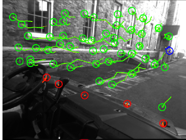
Fig. 1. Example of motion conflict: A moving camera in car sees static landmarks outside (green) with large optical flow and moving landmarks on the dashboard (red) with small optical flow. Each group of landmarks produce a different ego-motion estimate. Landmarks with noisy optical flow (blue) give incorrect ego-motion estimates.
